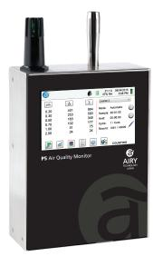
The Airy Technology Japan P5-301P and P5-501P Remote Particle Counters measure 0.3 or 0.5 to 25.0  $\mu$ m with a flow rate of 0.1 CFM (2.83 LPM) from an internal vacuum pump and are the most feature-advanced remote particle counters available. Integration is easy into a building automation and cleanroom management system via Ethernet, or (optional) Wireless 802.11 b/g, RS485 or RS232
